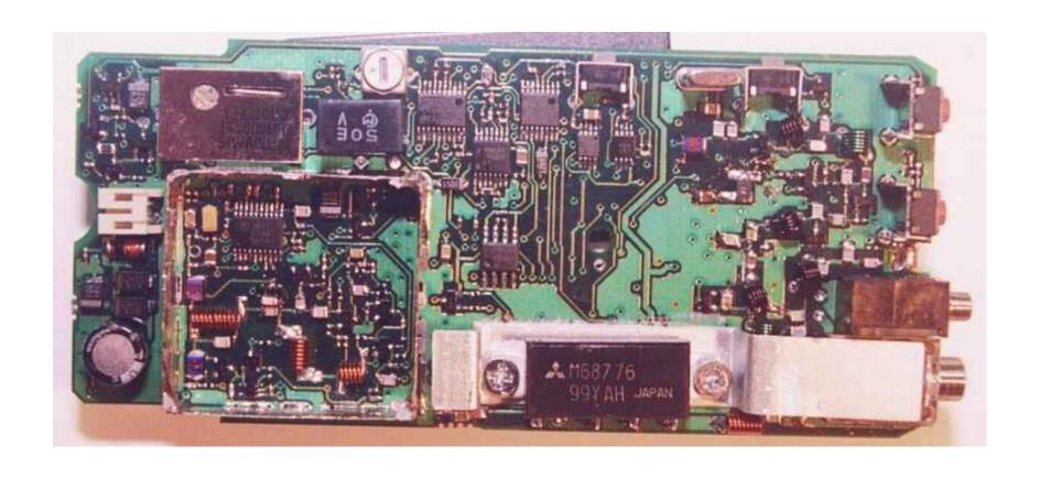
AIERIT13-144 SST-144 top side PCB assembly with VCO shield and speaker removed
