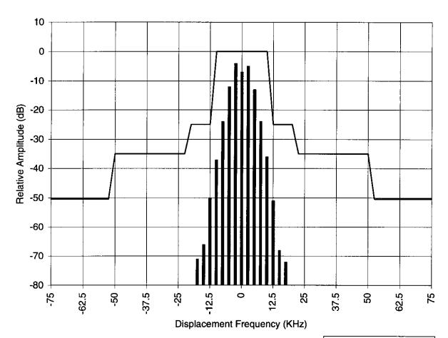
Channel Bandwidth: 25 KHz Power Output: 5.5 Watts 2500 Hz Sidebands
