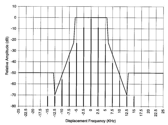
Channel Bandwidth: 12.5 KHz Power Output:
