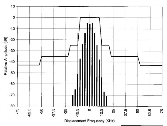
Channel Bandwidth: 25 KHz Power Output: 1.0 Watts 2500 Hz Sidebands
