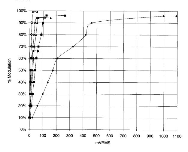
Channel Bandwidth: 12.5 KHz 100% Modulation: 2.5 KHz → 300 Hz → 500 Hz → 750 Hz → 1000 Hz → 2000 Hz → 3000 Hz TYPE OF TEST: PERCENT MODULATION VS. MODULATION INPUT VOLTAGE
