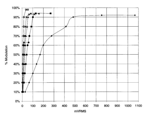
Channel Bandwidth: 12.5 KHz 100% Modulation: 5 KHz → 300 Hz → 500 Hz → 750 Hz → 1000 Hz → 2000 Hz → 3000 Hz
