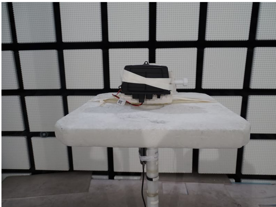
Photo 4: RSE setup 9 kHz to 30 MHz and > 1 GHz
