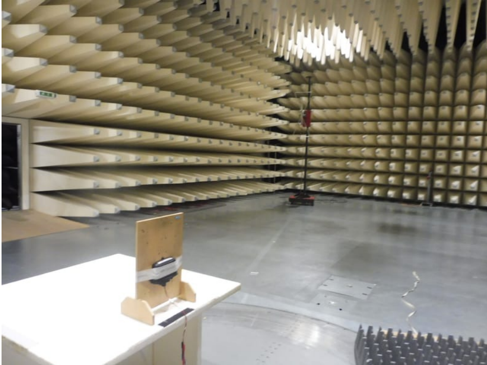
Photo 7: RSE setup 30 MHz to 1 GHz
