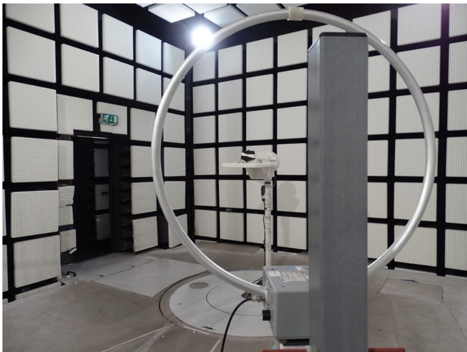
Photo 6: RSE setup 9 kHz to 30 MHz and > 1 GHz
