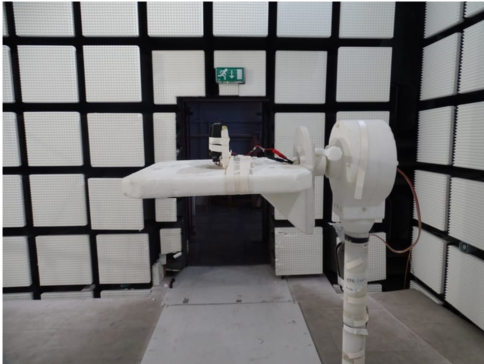
Photo 3: RSE setup 9 kHz to 30 MHz and > 1 GHz
