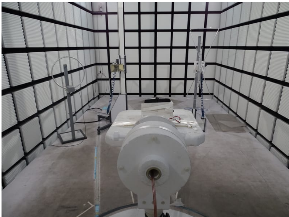
Photo 2: RSE setup 9 kHz to 30 MHz and > 1 GHz
