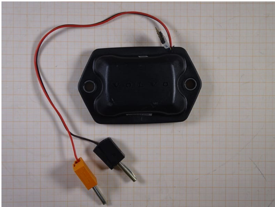
Photo 7: Modification for external power supply
