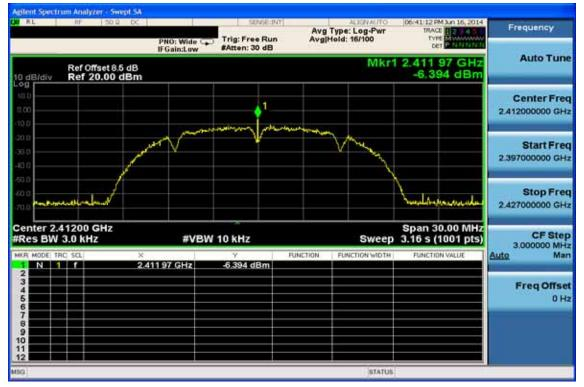
**Power Spectral Density Test Plot (CH-Mid)**
