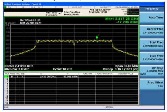
**Power Spectral Density Test Plot (CH-Mid)**
