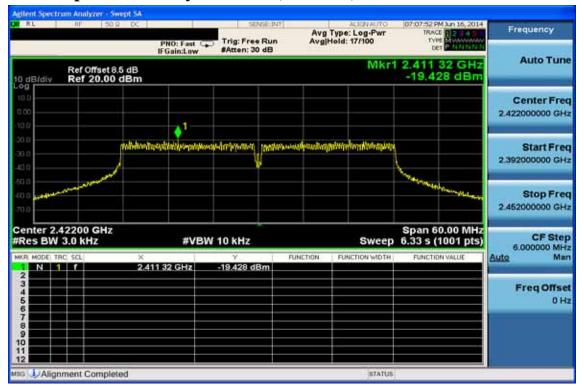
**Power Spectral Density Test Plot (CH-Mid)**
