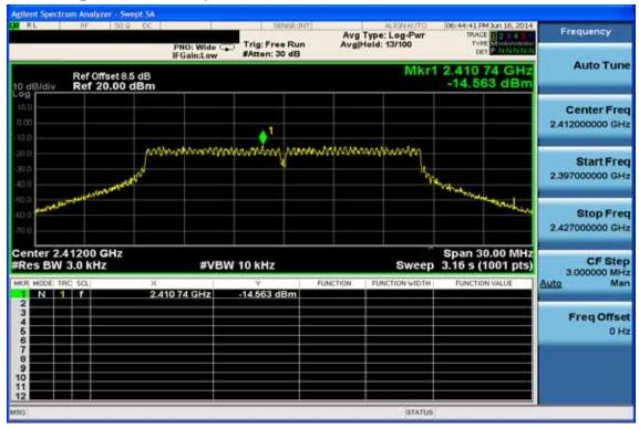
**Power Spectral Density Test Plot (CH-Mid)**
