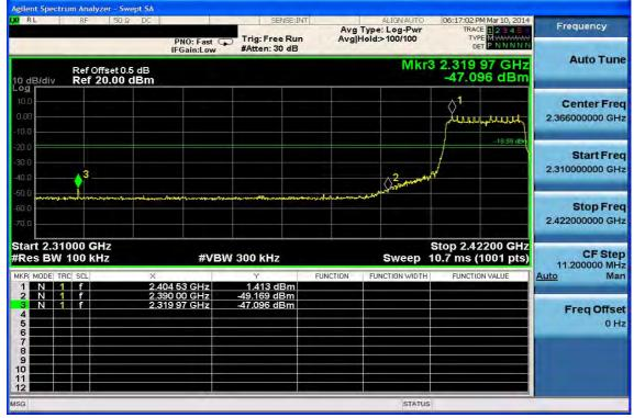
**Band Edges Test Data 2462MHz**
