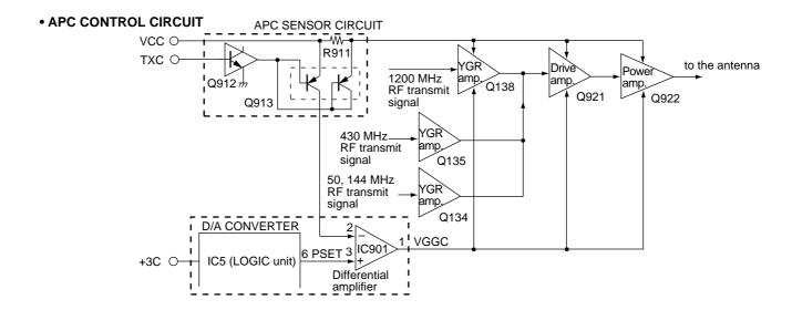
The APC sensor (R911) detects driving current from the drive voltage at the YGR (Q138), drive (Q921) and power (Q922) amplifiers. The detected current is converted into DC voltage at Q913, then applied to the APC control circuit (IC901, pin 2). The applied voltage is compared with a "PSET" voltage from the CPU via the D/A converter (LOGIC unit; IC5), and the APC control circuit outputs "VGGC" voltage from pin 1 to control the YGR, drive and power amplifiers.
