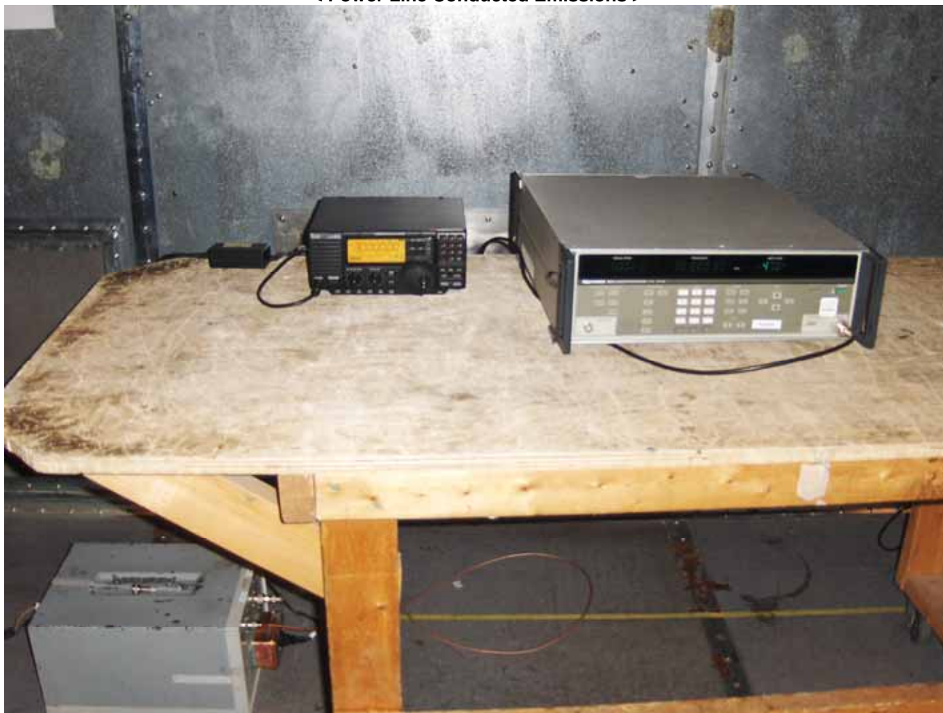
< Power Line Conducted Emissions >
