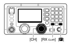
2 Rotate [CH] to improve the audio readability.Adjustable between ±150 Hz in 10 Hz steps.
