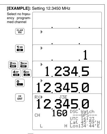
When push  $\frac{c_{LA}^{m}}{m}$  then rotate [CH] to re-select the channel, the set frequency will be cleared.
