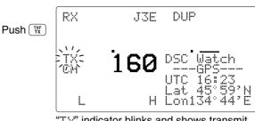
"TX" indicator blinks and shows transmit frequency.
