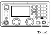
•The display shows the transmit frequency.
