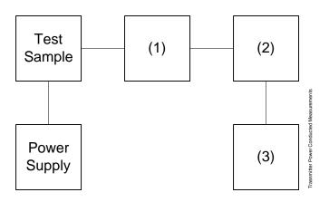
Asset Description s/n (as applicable) (1) COAXIAL ATTENUATOR i00122 Narda 766-10 7802 i00123 Narda 766-10 7802A i00069 Bird 8329 (30 dB) 1006 i00113 Sierra 661A-3D 1059 (2) POWER METERS i00014 HP 435A 1733A05836 i00039 HP 436A 2709A26776
