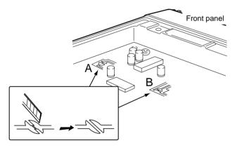
**NOTE:** Be sure to re-solder above disconnected points, otherwise no TX modulation or AF output is available when you remove the scrambler units.
