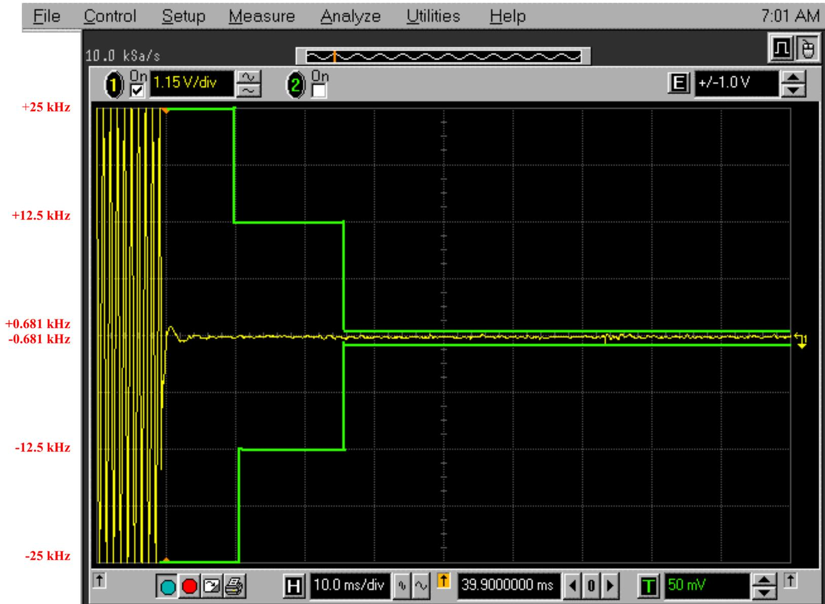
**Transient Frequency Behavior for 25 kHz Channel Spacing Operation**
