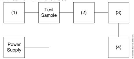
Asset Description s/n (as applicable) (1) AUDIO OSCILLATOR/GENERATOR i00010 HP 204D 1105A04683 i00017 HP 8903A 2216A01753 i00012 HP 3312A 1432A11250 (2) COAXIAL ATTENUATOR i00122 Narda 766-10 7802 i00123 Narda 766-10 7802A i00069 Bird 8329 (30 dB) 1006 i00113 Sierra 661A-3D 1059 (3) FILTERS; NOTCH, HP, LP, BP i00126 Eagle TNF-1 i00125 Eagle TNF-1 100-250 50-60 i00124 Eagle TNF-1 250-850
