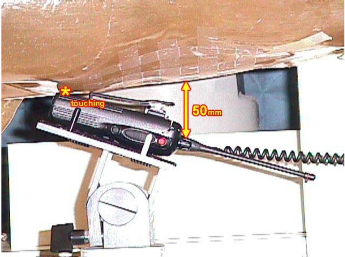
< Close-up view – Waist with the normal belt clip (M/N:MB-68) and the base of the EUT in contact with the phantom >
