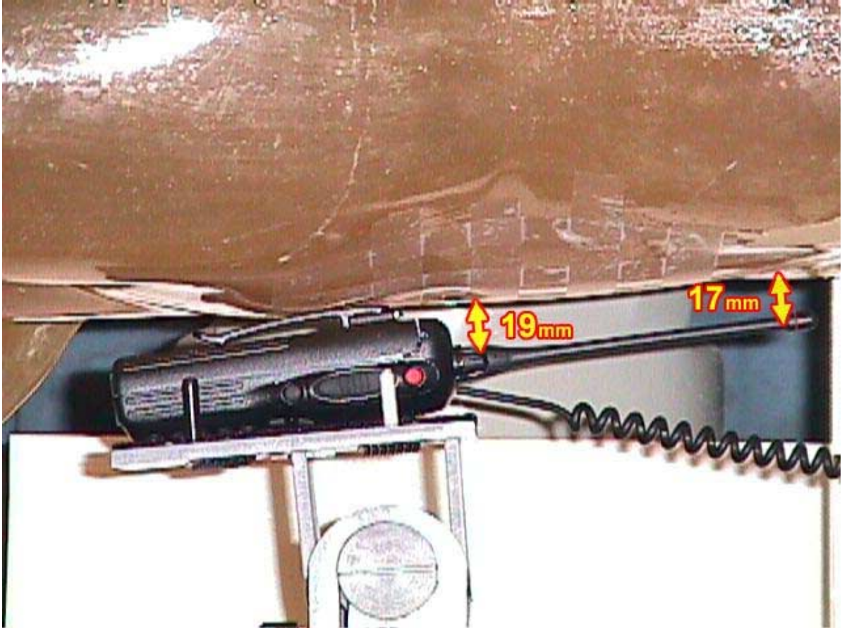
< Close-up view – Waist with the normal belt clip (M/N:MB-68) and the EUT parallel to the phantom >
