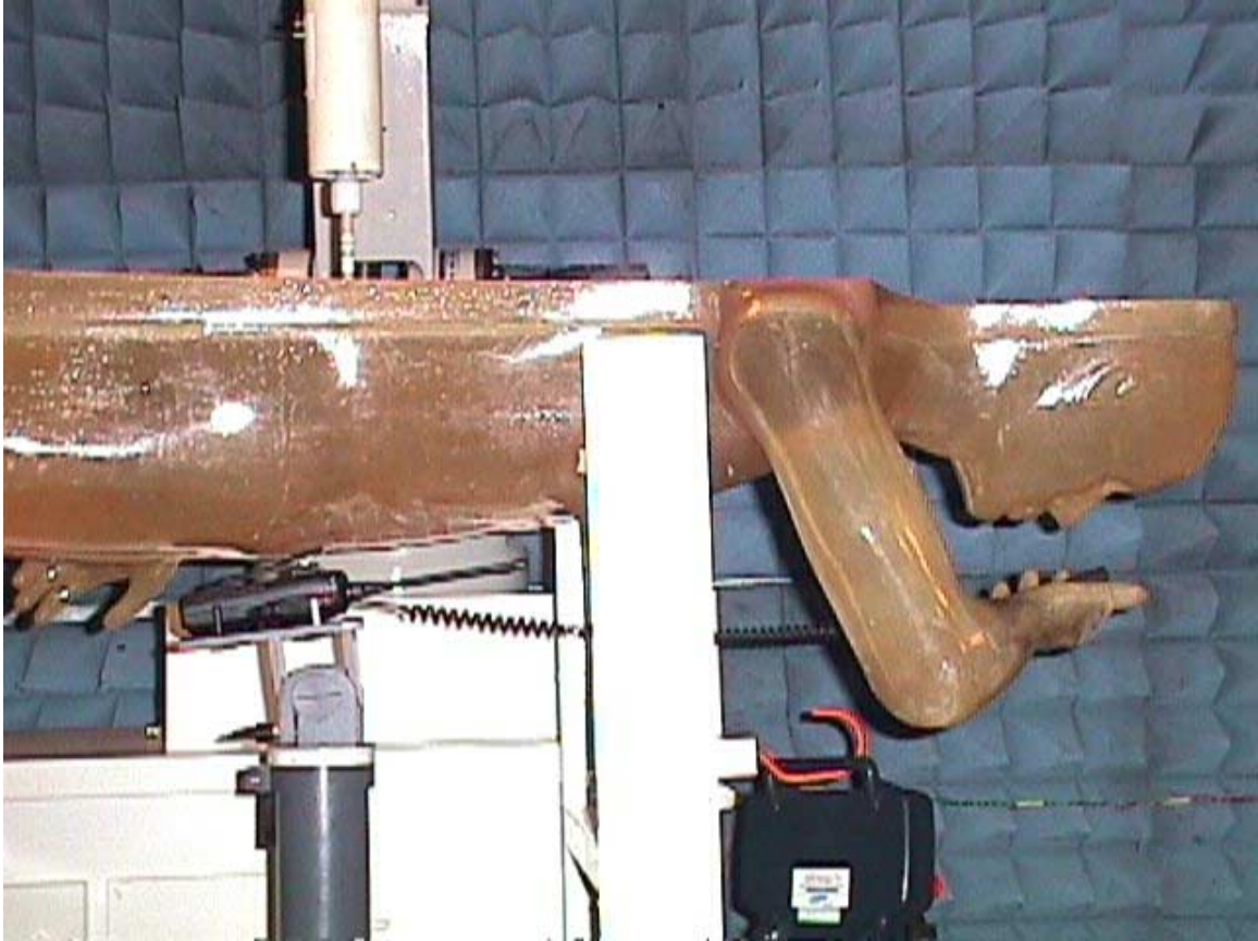
< Overview – Waist with the alligator belt clip (M/N:MB-74) and the EUT parallel to the phantom >
