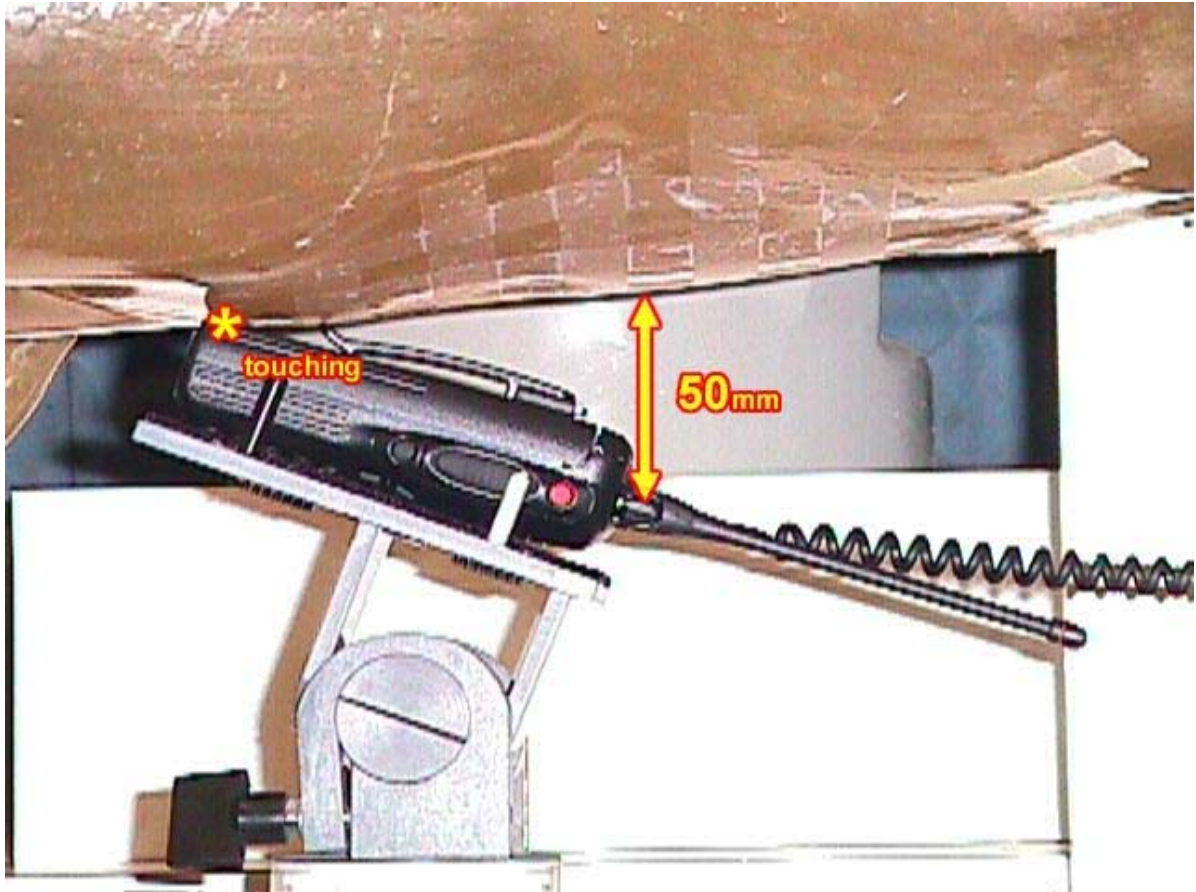
< Close-up view – Waist with the alligator belt clip (M/N:MB-74) and the base of the EUT in contact with the phantom >
