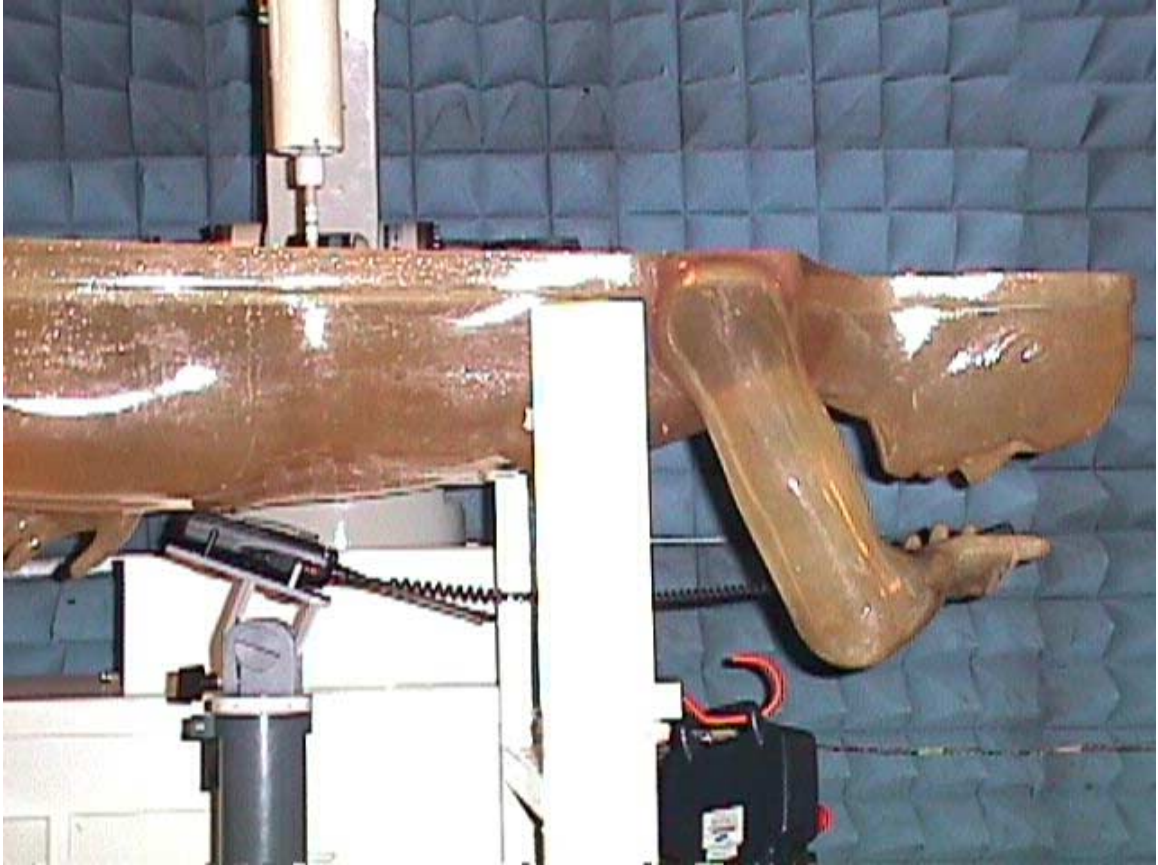
< Overview – Waist with the alligator belt clip (M/N:MB-74) and the base of the EUT in contact with the phantom >
