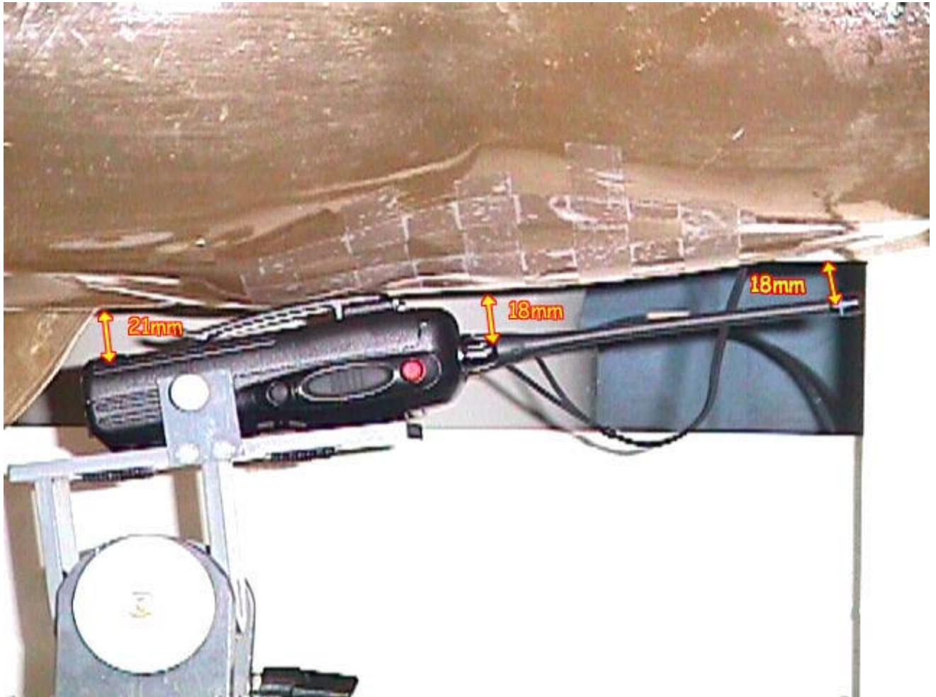
< Close-up view – Waist with the antenna positioned parallel to the phantom and the headset >
