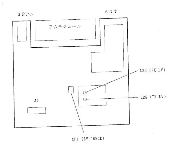
5-3 TRIMMER ADJUSTMENT for IC-F420 Select an operation using  $[\uparrow]/[\downarrow]$  keys, then set the specified value using  $[\leftarrow]/[\rightarrow]$  keys on the connected computer keyboard.
