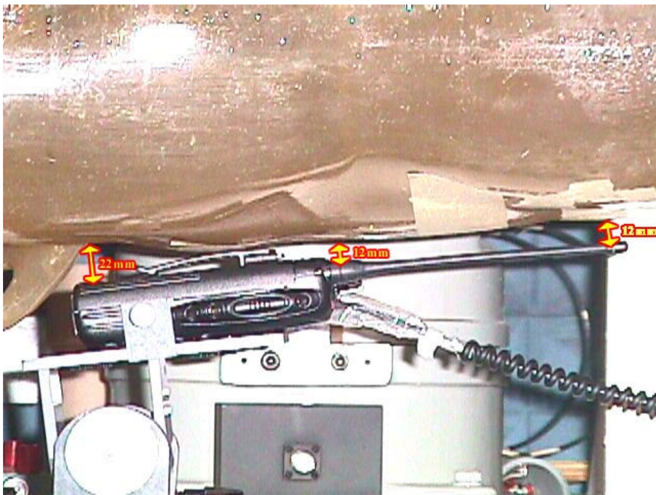
< Close-up view – Waist with the antenna positioned parallel with the phantom >
