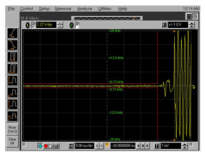
Plot # 21 Transient Frequency Behavior Carrier Frequency: 146.05 MHz, Wide Band (25 kHz Channel Spacing) Power: 5 Watts Modulation: FM with 2.5 kHz Sine Wave Description: Carrier On Time
