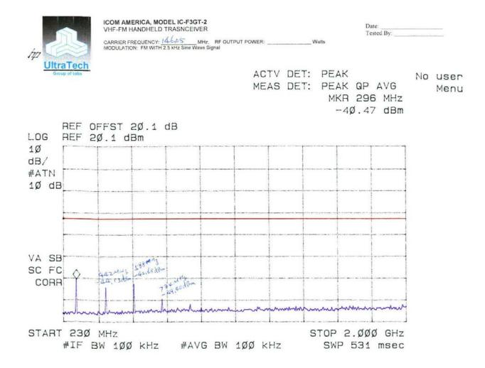
Plot #11 Spurious Emissions at Antenna Terminals Carrier Frequency: 160.05 MHz, Wide Band (25 kHz Channel Spacing) Power: 1 Watt Modulation: FM with 2.5 kHz Sine Wave
