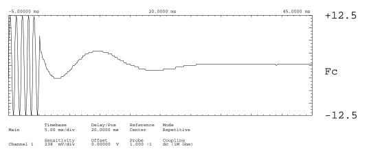
Trigger mode : Edge On Negative Edge Of Chan2 Trigger Level Chan2 = -8.500 mV (noise reject ON) Holdoff = 40.000 ns
