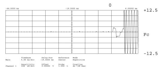
Trigger mode : Edge On Positive Edge Of Chan2 Trigger Level Chan2 = -175.000 mV (noise reject ON) Holdoff = 40.000 ns
