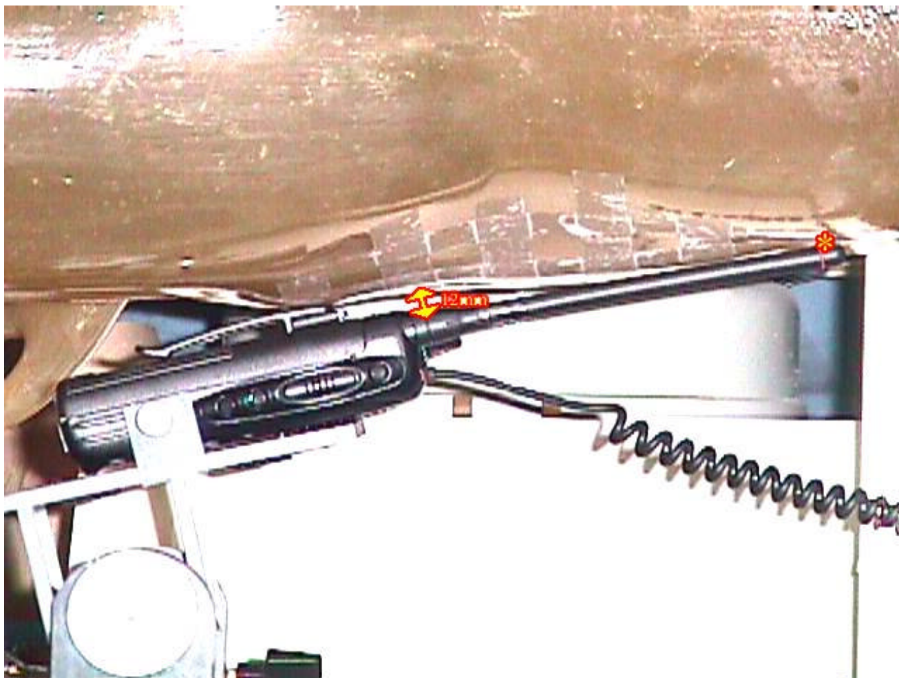
< Close-up view – Waist with normal belt clip and the antenna Touching the phantom >
