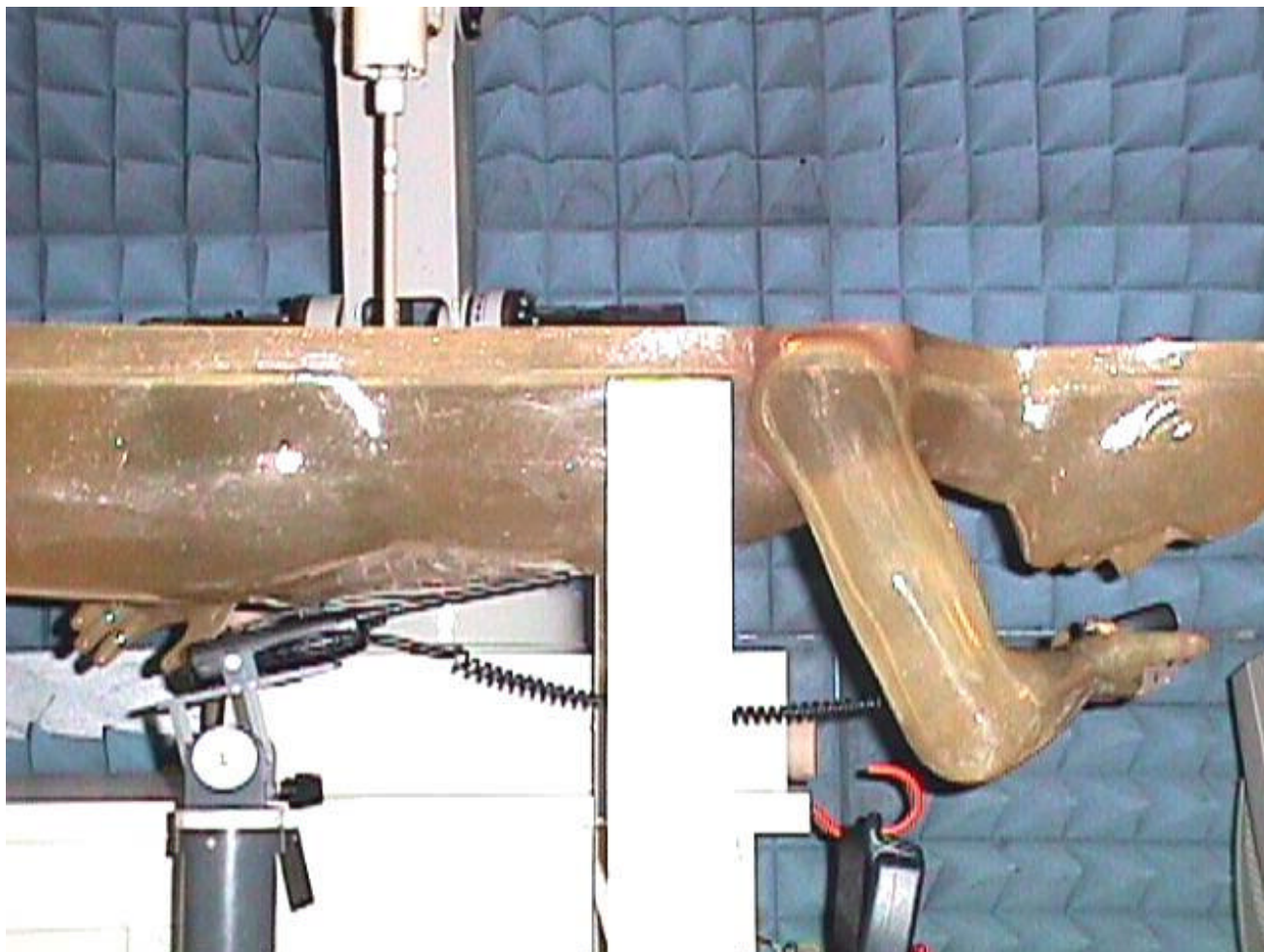
<Overview – Waist with normal belt clip and the antenna touching the phantom>
