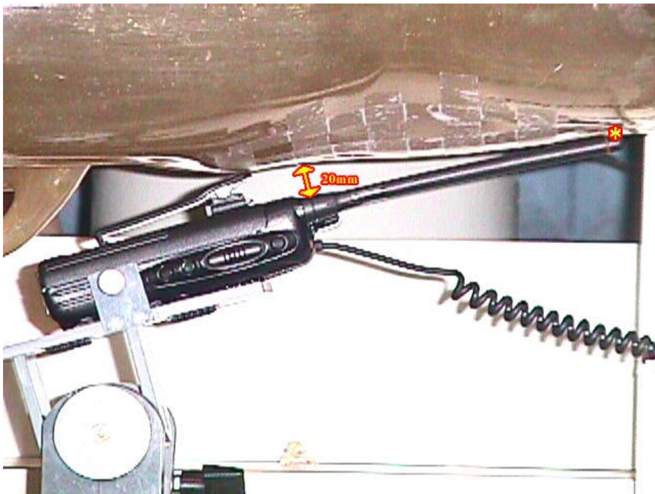
< Close-up view – Waist with alligator belt clip and the antenna touching the phantom >
