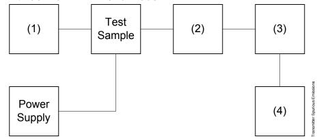
Asset Description s/n (as applicable) (1) AUDIO OSCILLATOR/GENERATOR i00010 HP 204D 1105A04683 i00017 HP 8903A 2216A01753 i00012 HP 3312A 1432A11250 (2) COAXIAL ATTENUATOR i00122 Narda 766-10 7802 i00123 Narda 766-10 7802A i00069 Bird 8329 (30 dB) 1006 i00113 Sierra 661A-3D 1059 (3) FILTERS: NOTCH, HP, LP, BP
