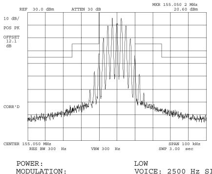
VOICE: 2500 Hz SINE WAVE MASK: B, VHF/UHF 25kHz, w/LPF
