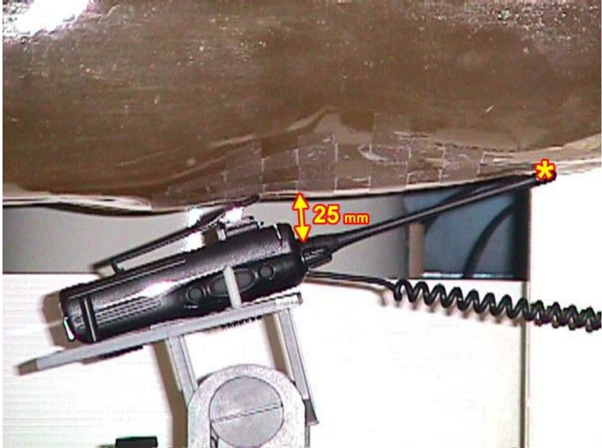
< Close-up view – Waist with the alligator belt clip (M/N:MB-74) and the tip of the antenna in contact with the phantom >
