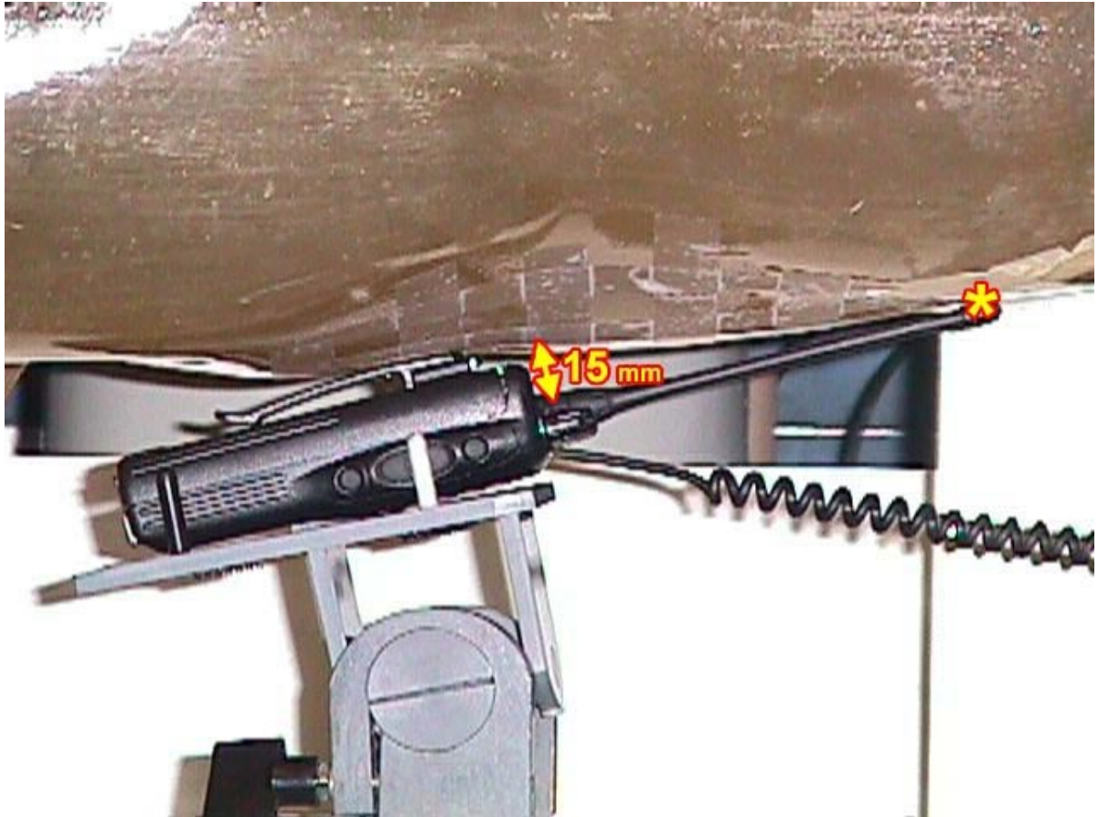
< Close-up view – Waist with the normal belt clip (M/N:MB-68) and the tip of the antenna in contact with the phantom >
