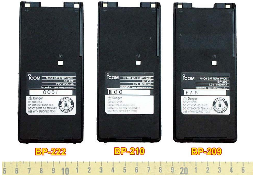
< Battery packs : BP-222 (600mAh), BP-210 (1650mAh), BP-209 (1100mAh) >
