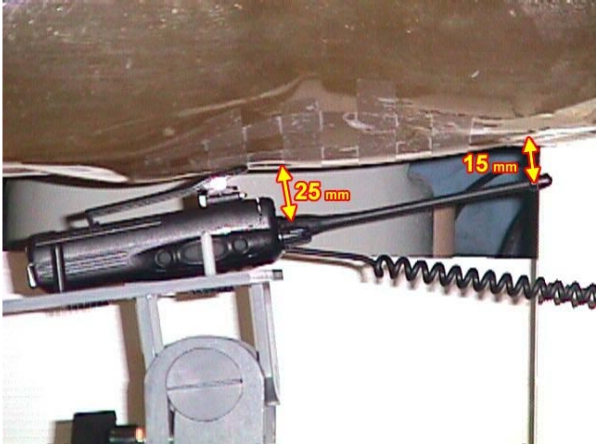
< Close-up view – Waist with the alligator belt clip(M/N:MB-74) and the EUT parallel to the phantom >
