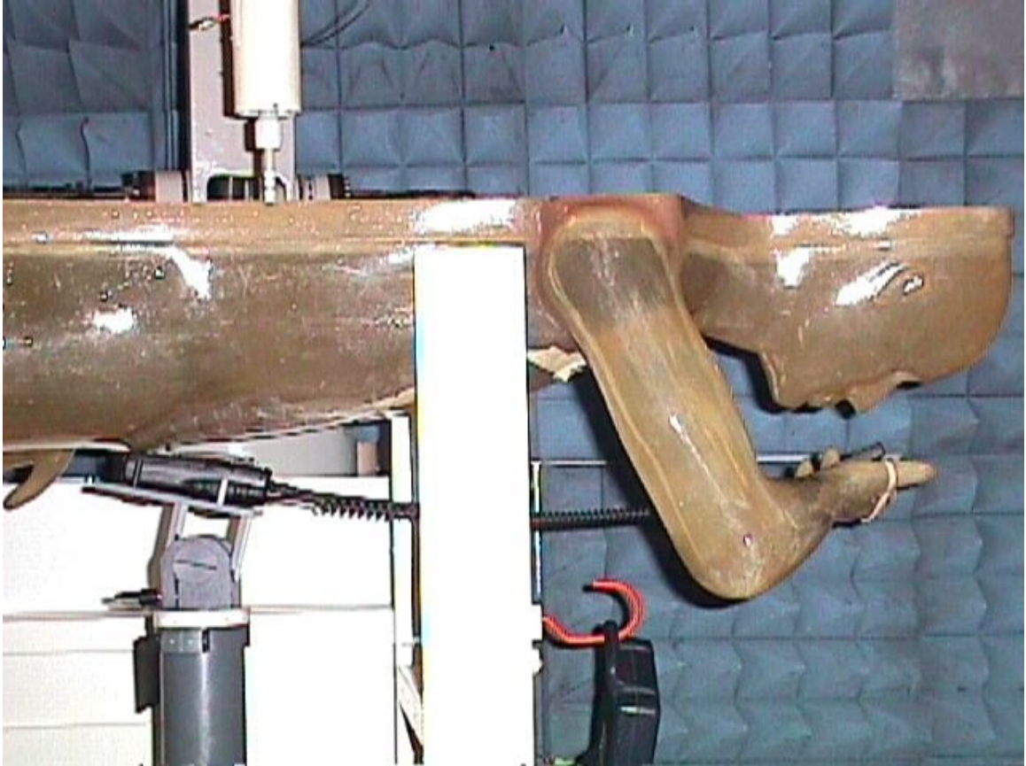
< Overview – Waist with the normal belt clip (M/N:MB-68) and the base of the EUT in contact with the phantom >
