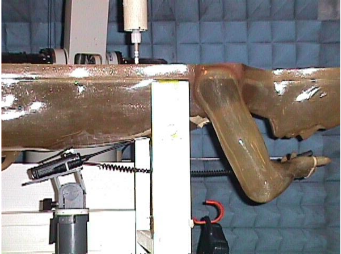
< Overview – Waist with the alligator belt clip (M/N:MB-74) and the tip of the antenna in contact with the phantom >
