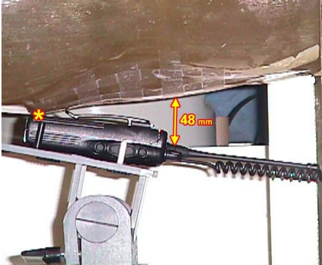
< Close-up view – Waist with the normal belt clip (M/N:MB-68) and the base of the EUT in contact with the phantom >
