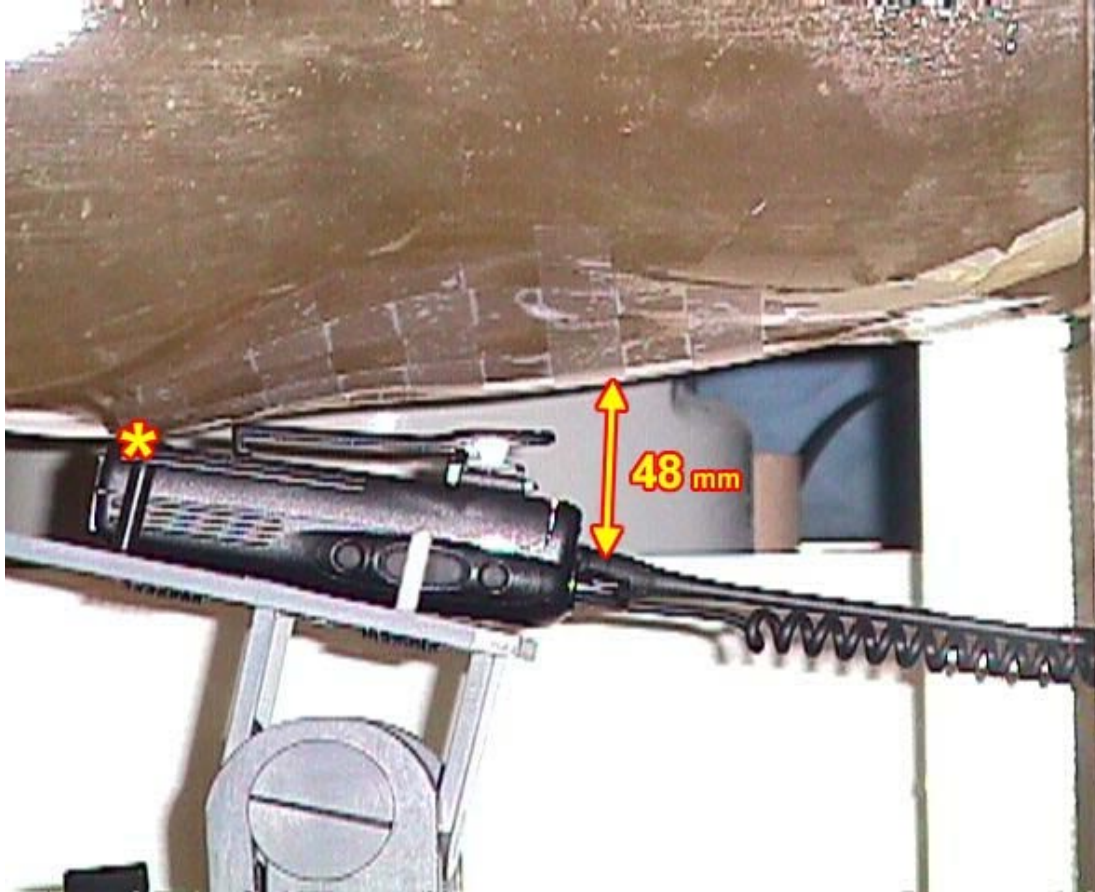
< Close-up view – Waist with the alligator belt clip (M/N:MB-74) and the base of the EUT in contact with the phantom >
