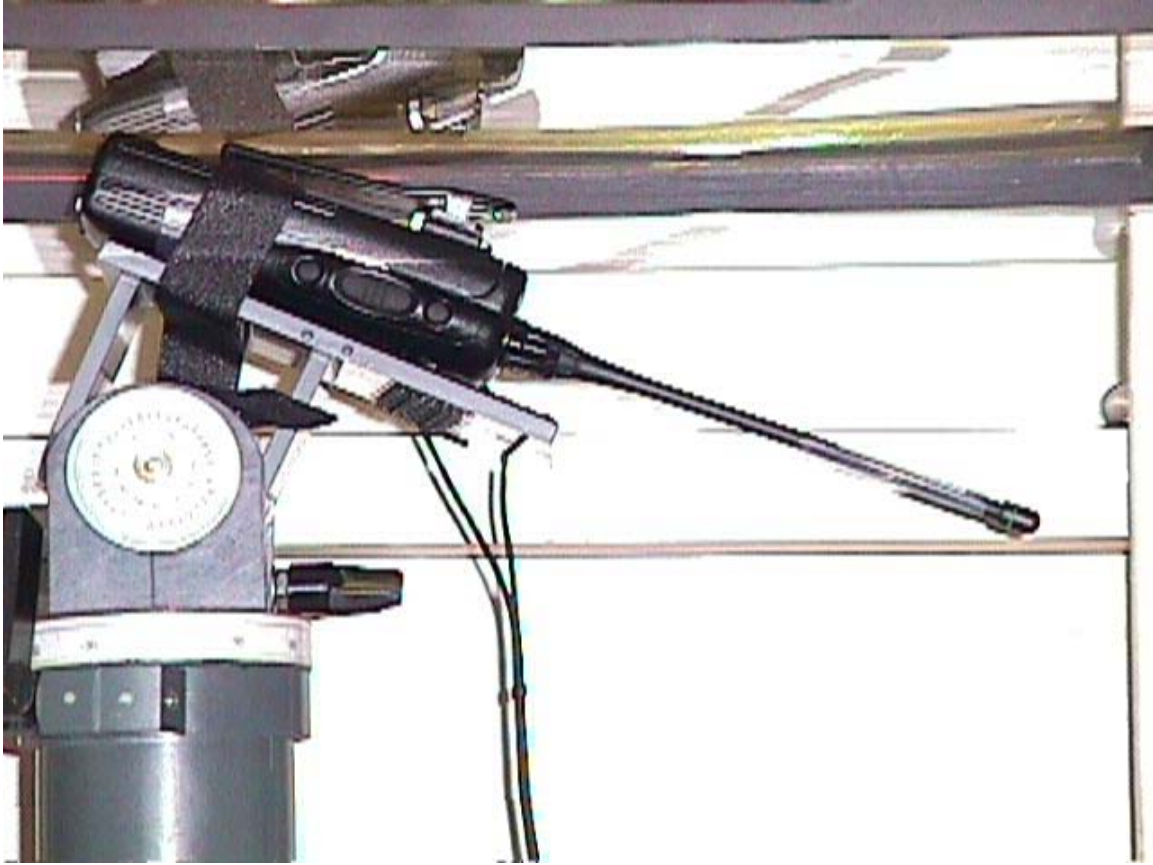
< The bottom of the EUT in contact with the phantom with the alligator belt clip(M/N: MB-74) and headset(M/N: HS-51) – Close-up View >
