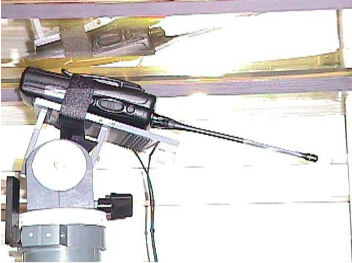
< The bottom of the EUT in contact with the phantom with the belt clip(M/N: MB-68) and headset(M/N: HS-51) – Close-up View >
