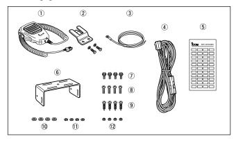
① Microphone ...... 1 6 Mounting bracket ...... 1 (2) Microphone hanger and (7) Bracket bolts ...... 4 8 Mounting screws (M5×12) . 4 screw set ...... 1 set (3) Microphone hanger cable . 1 9 Self-tapping screws (M5×20) 4 DC power cable (OPC-1132) .....4 (10) Flat washers ...... 4 ......1 (5) Function name stickers\* (1) Spring washers ..... 4 (KEY STICKER) .....1 12 Nuts ...... 4
