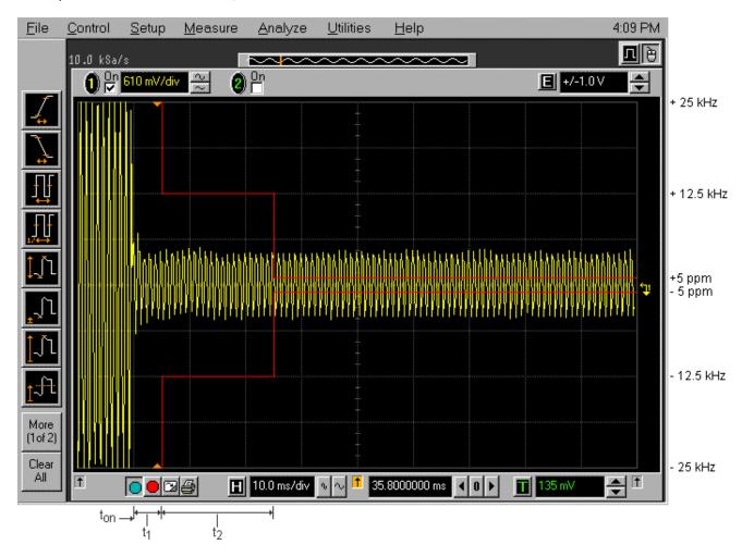
Carrier Frequency: 136.1 MHz Channel Spacing: 25 kHz
