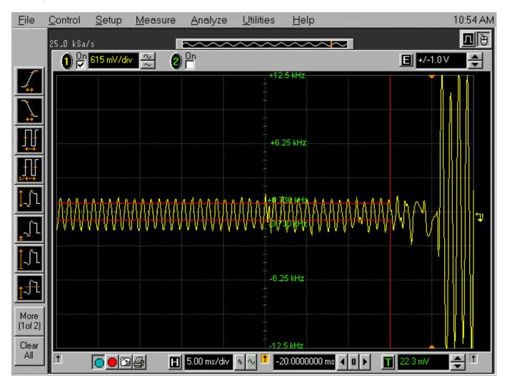
Plot # 29 Transient Frequency Behavior Carrier Frequency: 146.05 MHz, WB (25 kHz Channel Spacing) Power: 5 W Modulation: Unmodulated Description: Carrier On Time
