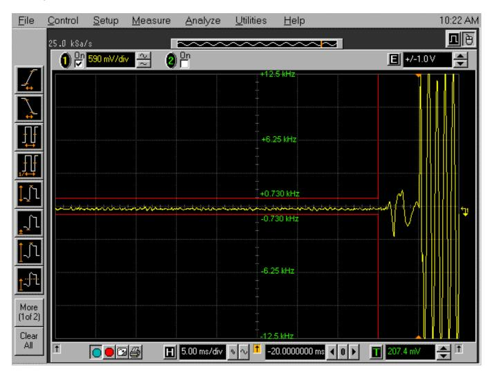
Plot # 27 Transient Frequency Behavior Carrier Frequency: 146.05 MHz, NB (12.5kHz Channel Spacing) Power: 5 W Modulation: FM with 2.5 kHz Sine Wave Description: Carrier On Time
