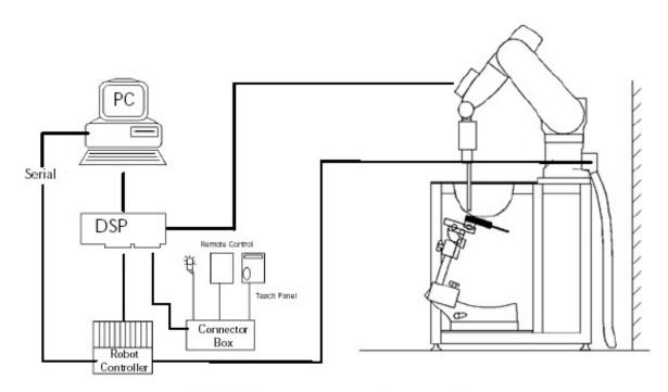
Figure 2.1 SAR Measurement System Setup
