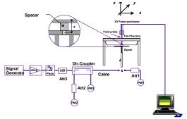
Figure 7.1 Dipole Validation Test Setup
