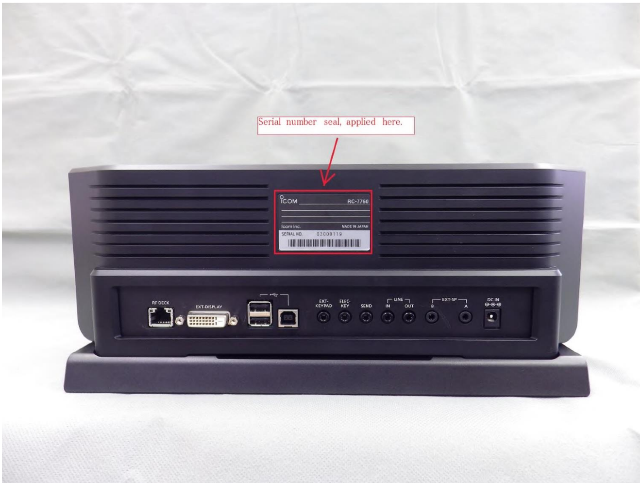
Controller Serial number seal location
