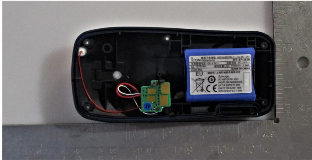
<Li-ion Chargeable Battery (BP-282N, 3.6V, 1570mAh)>
