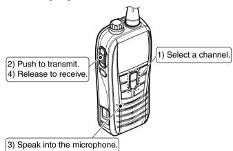
IMPORTANT: To maximize the readability of your transmitted signal, pause for a second after pushing [PTT], hold the microphone 5 to 10 cm (2 to 4 inches) from your mouth and speak at a normal voice level.
