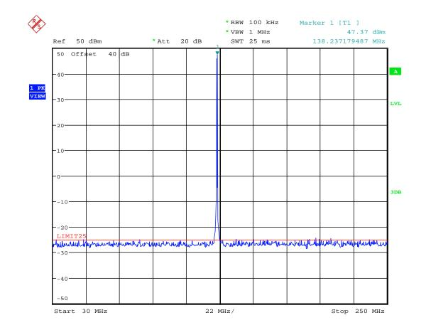
5.9.3.1. Configuration: Tx Conducted, 138.1MHz, 6.25 KHz, Digital, High power
