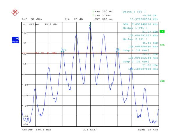
**5.8.3.2. Configuration: 99% OBW, 138.1MHz, 12.5 KHz, Analog, High power** OBW: 10.376 KHz
