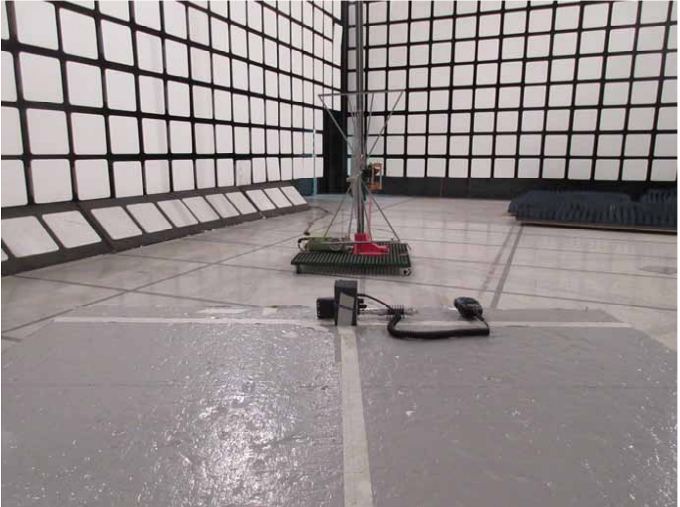
Radiated Emissions at 3 m
