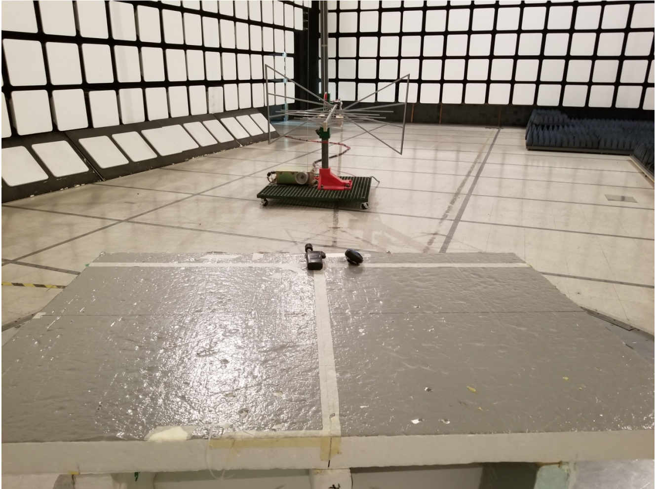
Radiated Emissions at 3 m, 30 - 1000 MHz Orthogonal Position 1
