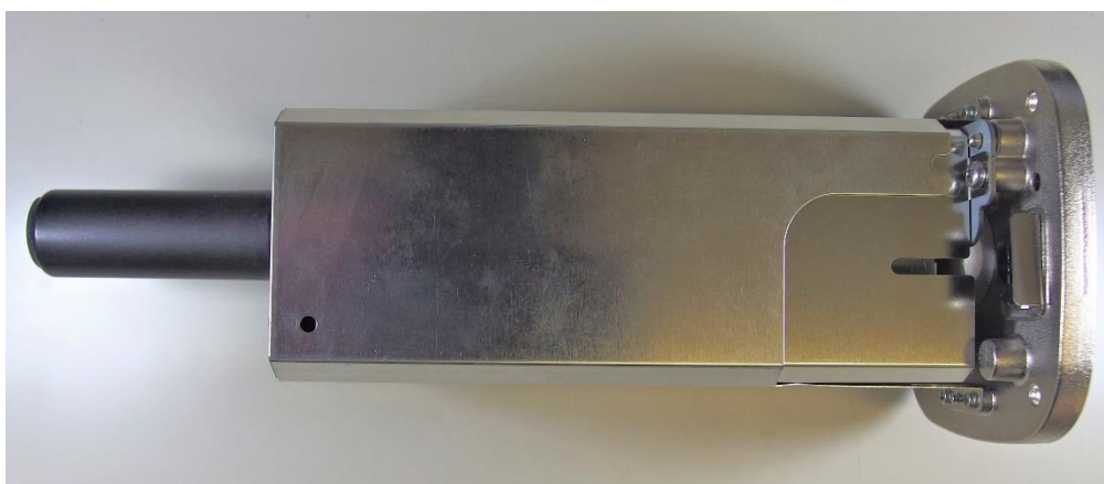
AH-41 RX Unit with chassis, antenna and shield Side B
