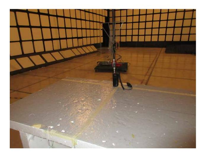
Radiated Emission at 3m (Orthogonal Position 1)
