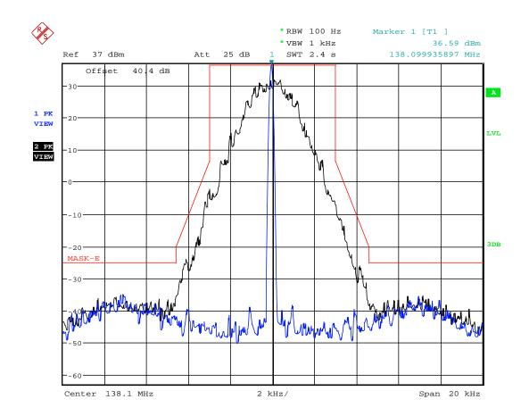
5.8.3.34. Configuration: Mask E, 138.1MHz, 6.25 KHz, Digital, Low power
