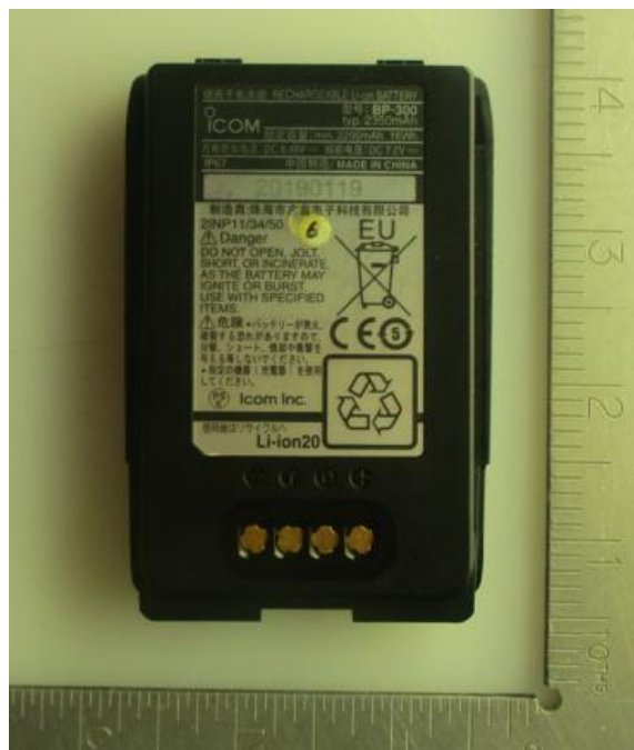
Li-ion Chargeable Battery (M/N: BP-300, 7.2V, 2350mAh)
