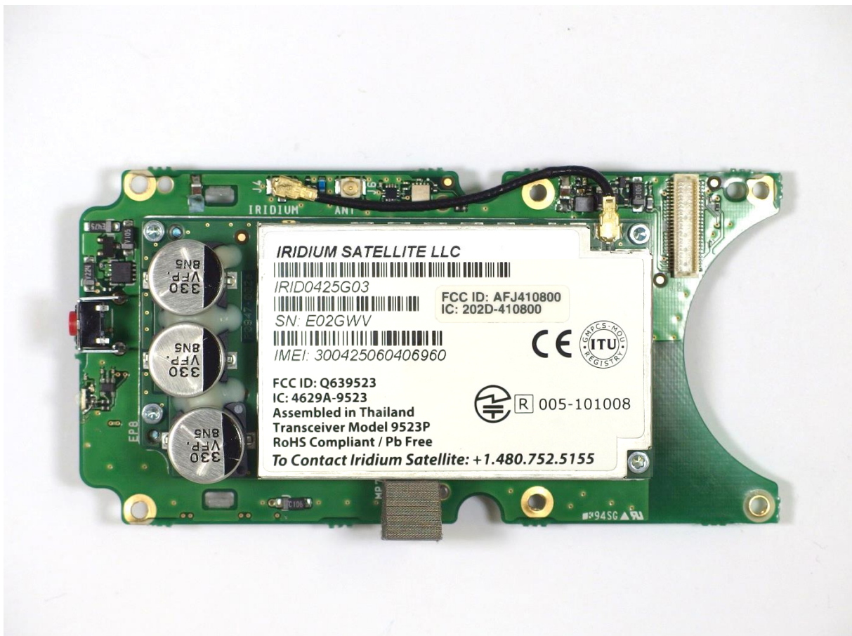
FRONT UNIT with IRIDIUM MODEM attached (SIDE B)
