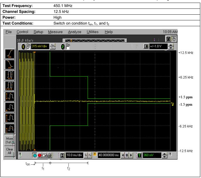
Plot 5.12.3.2. Transient Frequency Behavior for 12.5 kHz Channel Spacing
