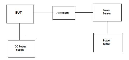
**TEST SETUP AND EQUIPMENT LIST**
