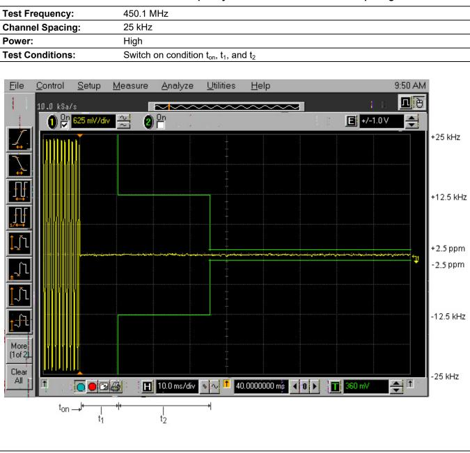
Plot 5.12.3.4. Transient Frequency Behavior for 25 kHz Channel Spacing
