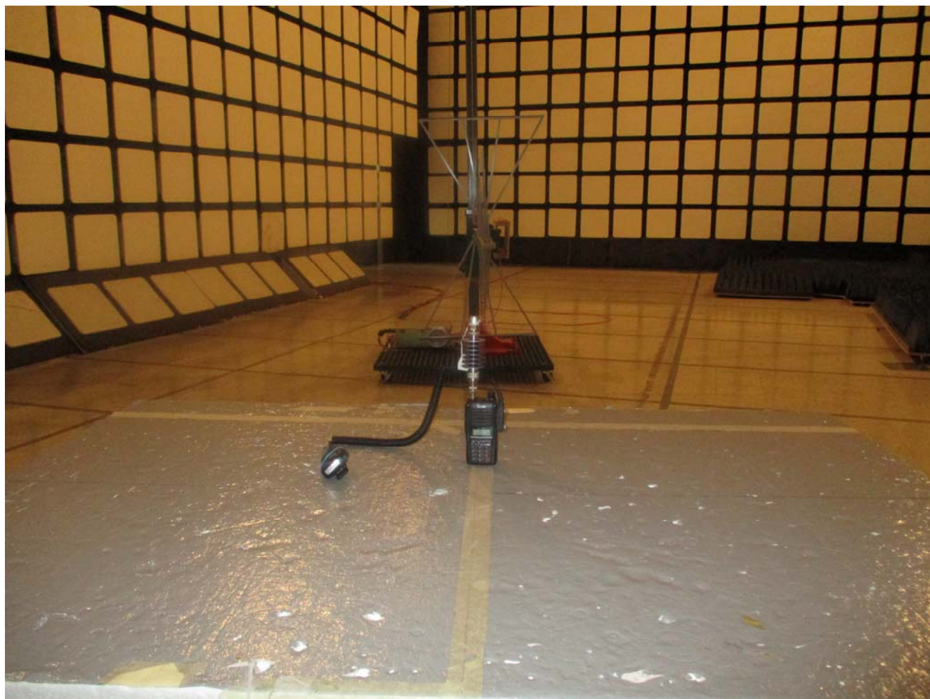
Radiated Emissions at 3 m, 30 - 1000 MHz Orthogonal Position 1
