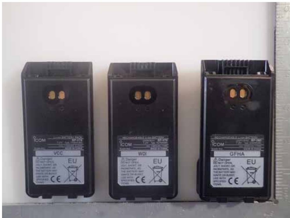
<Li-ion Chargeable Batteries (M/N:BP-278(1190mAh),BP-279(1570mAh),BP-280(2400mAh)>
