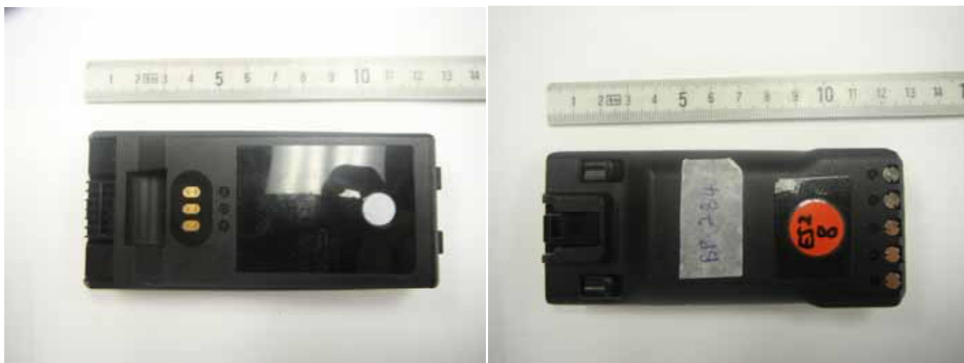
Li-ion Chargeable Battery (M/N: BP-284 Li-ion, 7.2V, 3210mAh)
