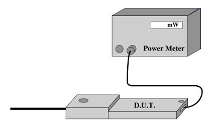
Power measurement is performed before and after the SAR to verify if the battery was delivering full power at the time of testing. A difference in output power would determine a need for battery replacement and to repeat the SAR test.
