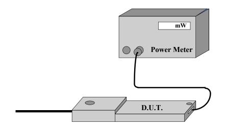
Power measurement is performed before and after the SAR to verify if the battery was delivering full power at the time of testing. A difference in output power would determine a need for battery replacement and to repeat the SAR test.
