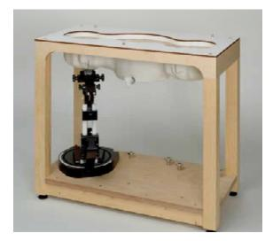
For Head mounted devices placed next to the ear, the phantom used in the evaluation of the RF exposure of the user of the wireless device is an IEEE P1528 compliant SAM Twin phantom, shaped like a human head and filled with a mixture simulating the dielectric characteristics of the brain. A left sided head and a right head are evaluated to determine the worst case orientation for SAR.
