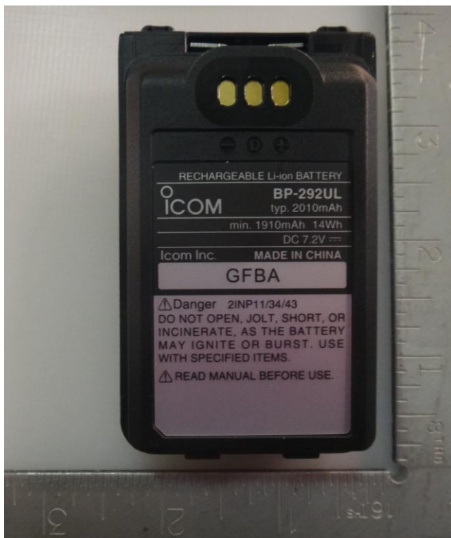
Li-ion Chargeable Battery (M/N: BP-292UL, 7.2V, 2010mAh)
