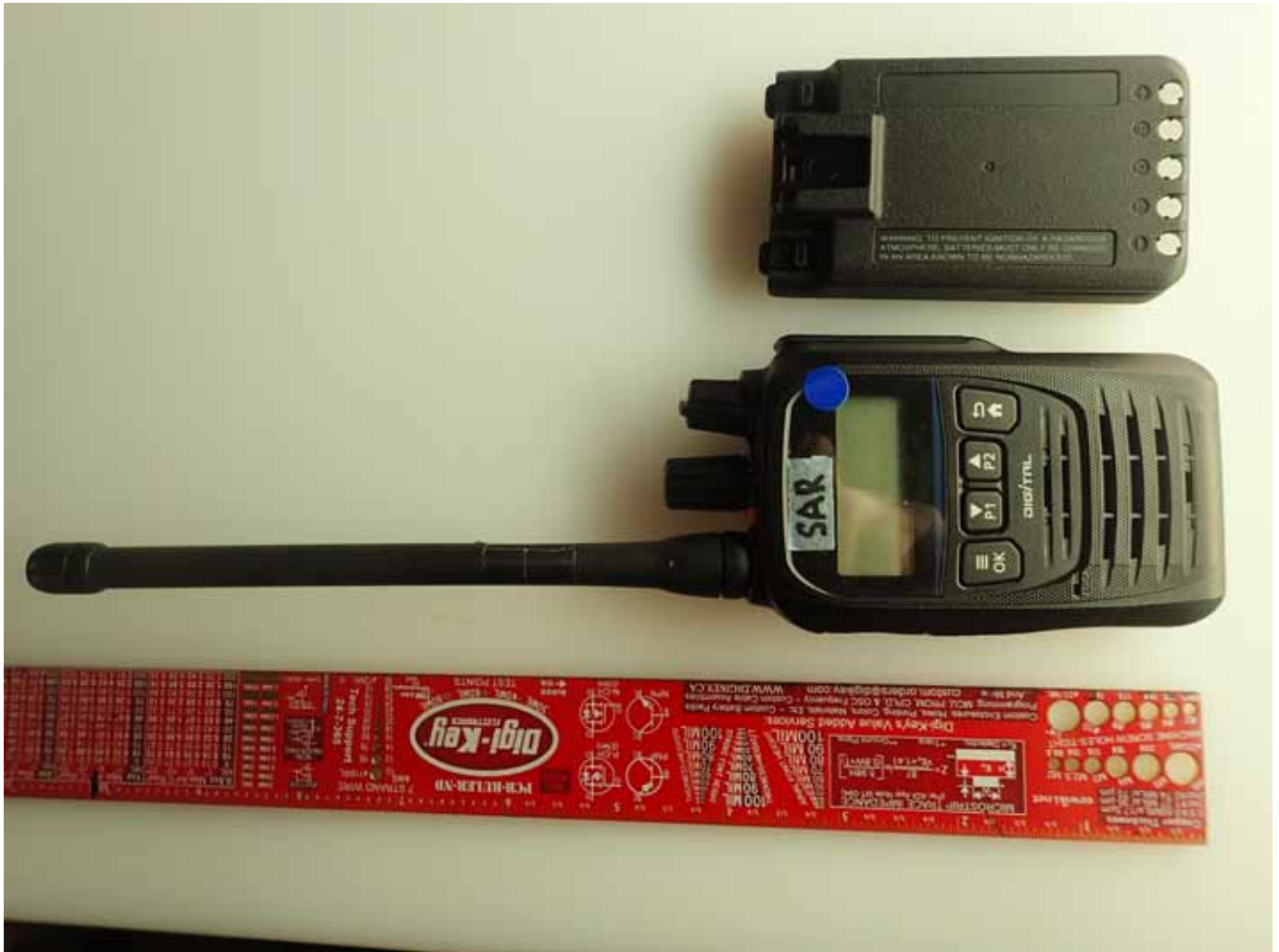
< D.U.T.'s front view with battery and FA-S61VC Cut Antenna 155MHz 151mm >
