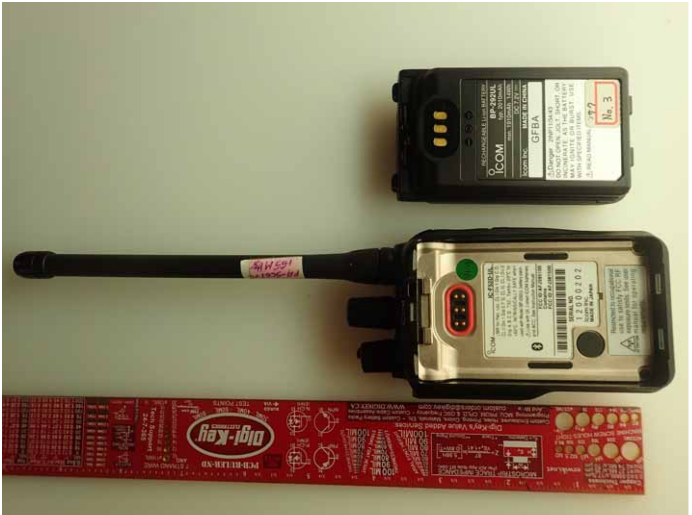
< D.U.T.'s rear view without battery and and FA-S61VC Cut Antenna 155MHz 151mm >
