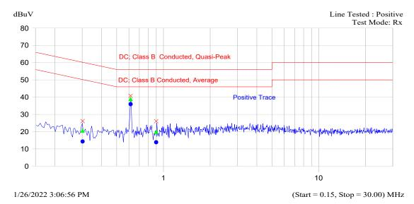
Frequency Avg Avg-Avg Limit Peak QP **Qp-Qp Limit Trace Name** dBuV dB MHz dBuV dBuV dB 0.615 40.8 38.9 35.9 -10.1 Positive Trace -17.1
