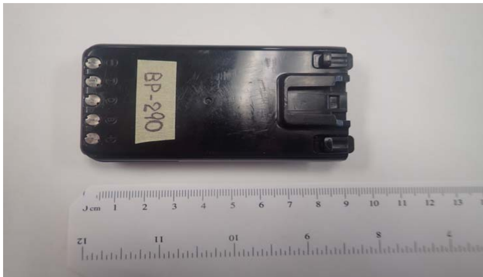
Li-ion Chargeable Battery (M/N: BP-290 Li-ion, 3.7V, 1960mAh)
