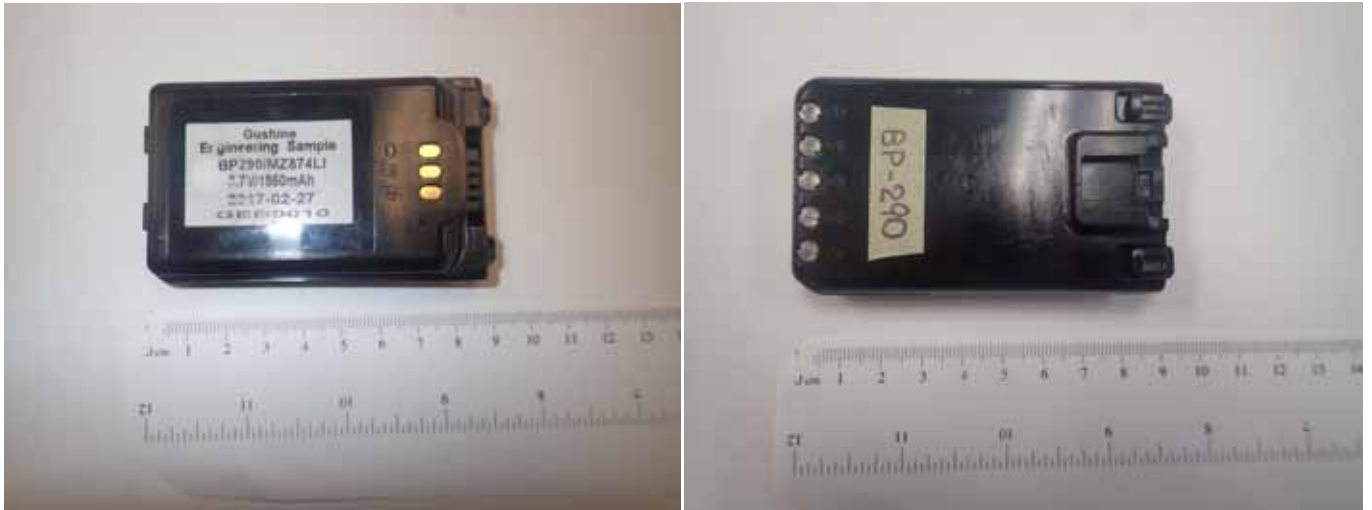
CHARGEABLE BATTERY (M/N: BP-290, 3.7V, 1950MAH)
